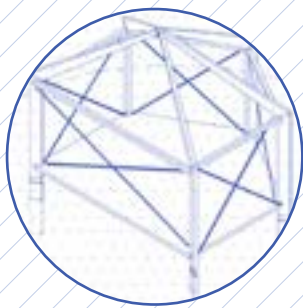
Steel Structure and Cross bracing for high wind speed.
