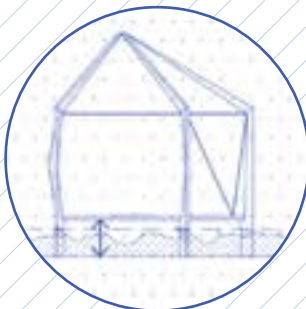
Adjustable floor level for flood (hydraulic).
