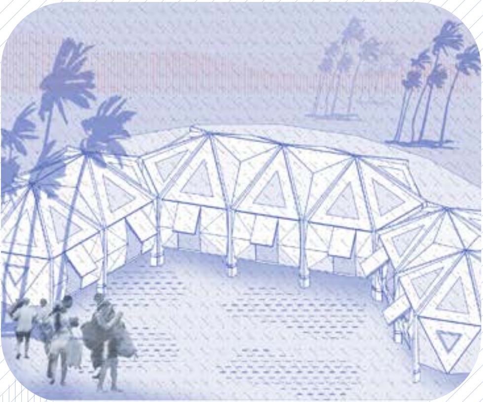
Foldable prefabricated wall and roof (air-tight for fire).
